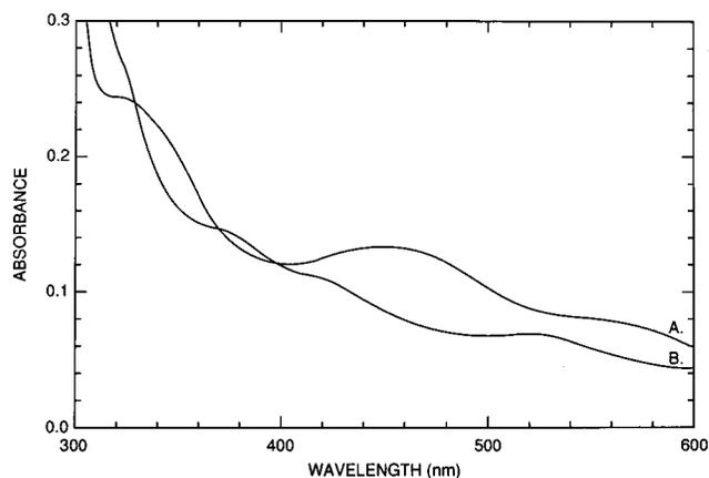
FIG. 3. Absorption spectra of ISP<sub>BPH</sub> (2.08 mg of protein per ml in a 1-ml total volume). (A) Oxidized; (B) reduced with NADPH in the presence of catalytic amounts (50  $\mu$ g each) of reductase<sub>BPH</sub> and ferredoxin<sub>BPH</sub>.
