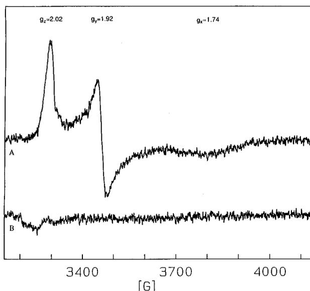
FIG. 4. EPR spectra of ISP<sub>BPH</sub> (1.2 mg of protein; 7.8 mg/ml). (A) Reduced with sodium dithionite; (B) oxidized.
