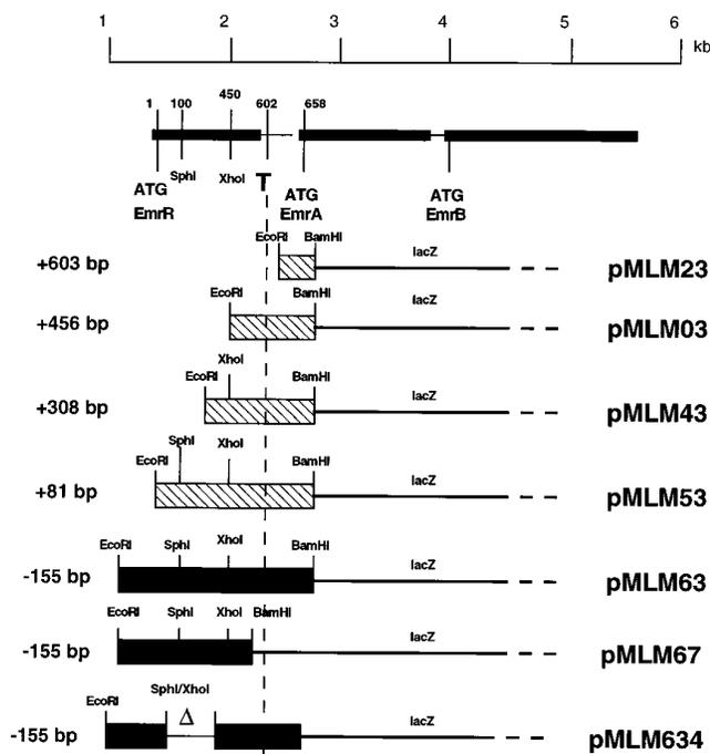
FIG. 1. Schematic representation of the cloned *emr-lacZ* fusions. The various fusions were constructed in the transcriptional vector pRS415 (35). *emr* sequences are shown as black and striped boxes for productive and nonproductive fusions, respectively. Numbers are given relative to the *emrR* translational start site and represent the 5' end of the DNA fragment in the individual fusions. The dashed vertical line shows the position of the terminator.
