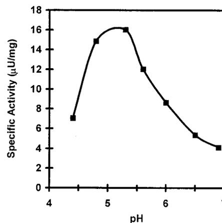
FIG. 5. Effect of pH on the activity of purified *S. solfataricus* HMG-CoA reductase. Assays of HMG-CoA reductase activity of the red fraction were conducted at the indicated pH, but under otherwise standard conditions.
