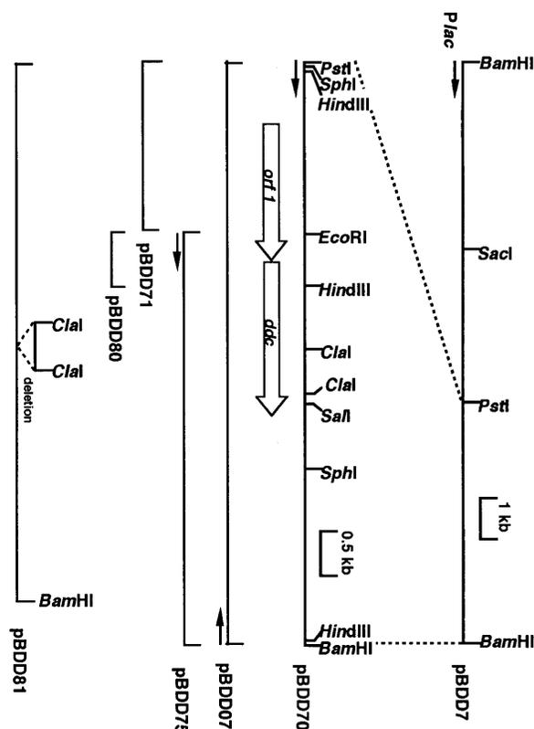
FIG. 1. Restriction map of the plasmids, constructed from the 14-kbp insert of pBDD7 containing *A. baumannii* ORF1 (*dat*) and *ddc* (19) used in this study. The relevant restriction sites are shown, and relative positions and directions of transcription of ORF1 (*dat*) and *ddc* are indicated by open arrows. The relevant plasmid inserts are shown diagrammatically, and the direction of the external *lacZ* transcription, where relevant, is indicated by filled arrows.
