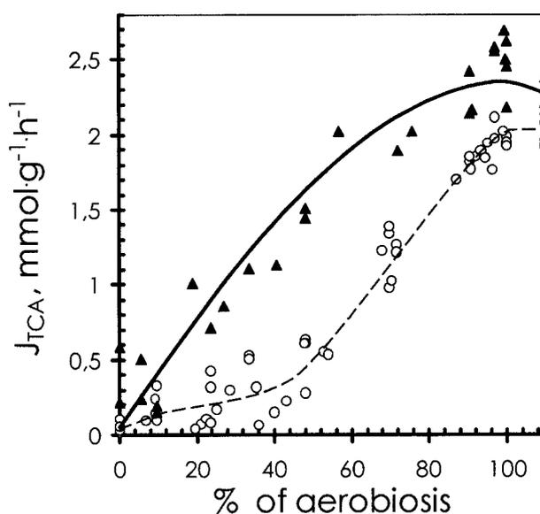
FIG. 4. Effect of the oxygen supply rate on the in vivo TCA cycle activities in the wild-type (open symbols) and  $\Delta arcA$  (filled symbols) strains. Data for the wild-type strain are derived from reference 1.
