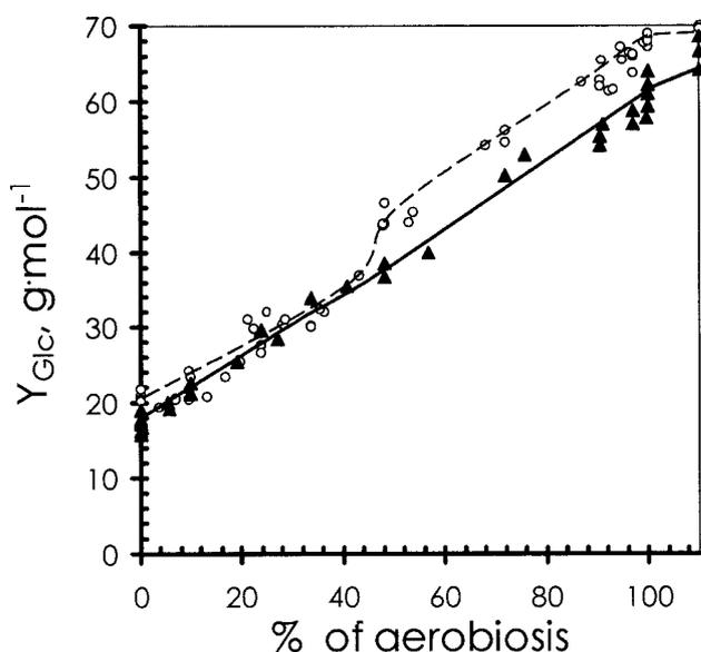
FIG. 1. Effect of the oxygen supply rate on the yield value for glucose ( $Y_{\text{glc}}$ , calculated as grams of dry weight formed per gram of glucose consumed and expressed as a percentage) in the wild-type (open symbols) and  $\Delta arcA$  (filled symbols) strains.
