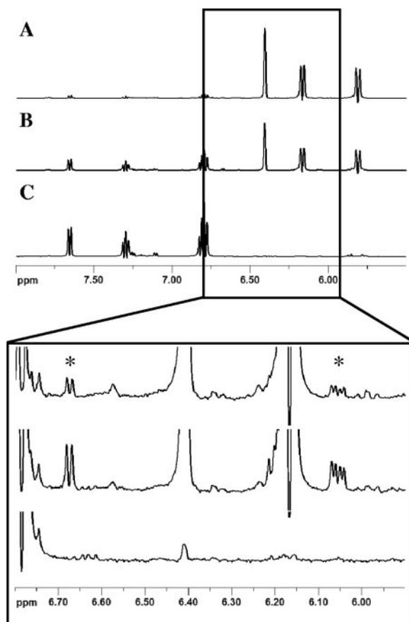
FIG. 4.  $^1\text{H}$  NMR spectroscopic time course analysis of the Irp9 reaction at  $10^\circ\text{C}$  using 5  $\mu\text{M}$  Irp9 and 2 mM chorismate after 3 min (A), after 22 min (B), and at completion after 90 min (C). Panels A to C show chorismate turnover into salicylate. The 5.9- to 6.8-ppm region is highlighted in the lower panel to show the formation of isochorismate. Peaks for isochorismate are indicated by asterisks.
