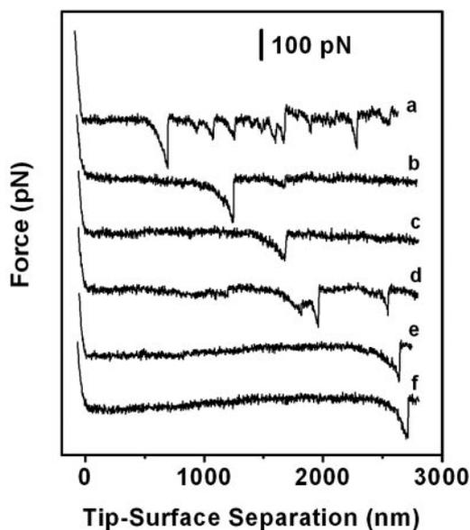
FIG. 5. (A) Collection of force spectra (retraction) taken with bacterium-coated tips over mica surfaces. Tip retraction speeds were 3  $\mu\text{m/s}$ , and the spectra from a to f were arranged in order of increasing retraction distance needed to apply tension on the pili.
