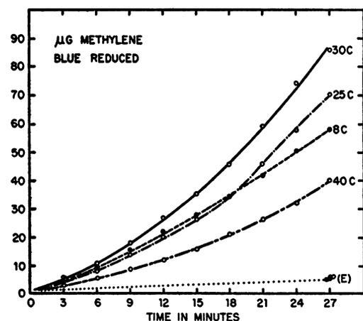
Figure 2. Micrograms of methylene blue reduced at 30 C after different periods of time by 2 mg of lyophilized (10-day) cells of *E. coli* which 30 minutes previously had been subjected to a pressure of 600 atm for 4 hours at 8, 25, 30, or 40 C. The upper four curves represent activity with succinate as the hydrogen donor; the dotted line (E) at the bottom represents endogenous activity with no succinate added.
